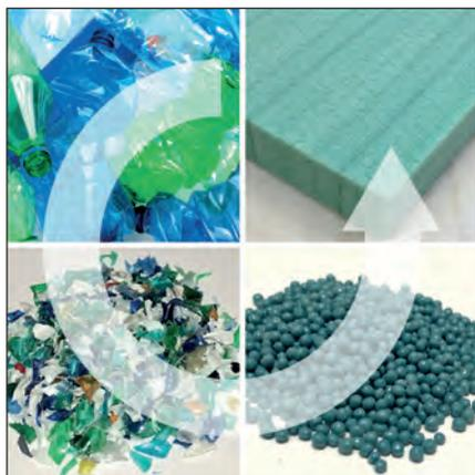
Cores in a sandwich construction are specified by designers and architects to increase stiffness and reduce the weight of the whole composite structure. Gurit has a range of core materials to fit any specification or manufacturing process.
