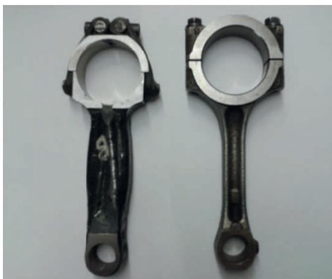
Fig. 3 - Example of a prototype of composite conrod (left) compared the traditional metal conrod (right)
