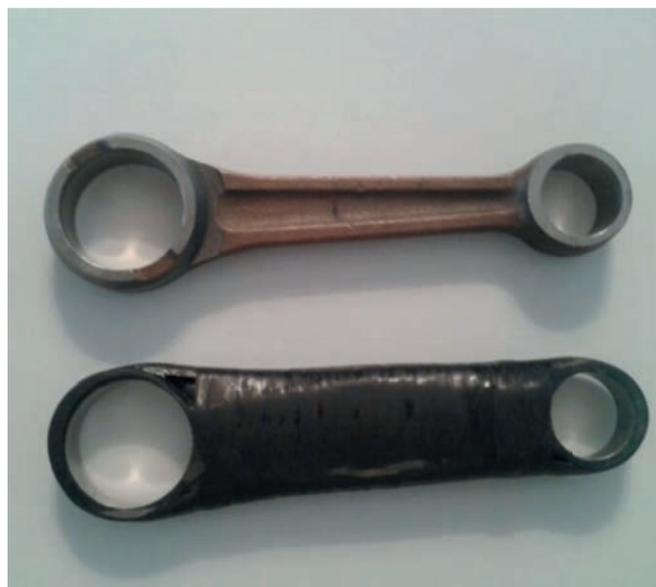
Fig. 1 - Metal traditional conrod (up), compared to composite conrod (down)
