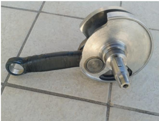
Fig. 2 - Composite conrod mounted on the scooter shaft.
