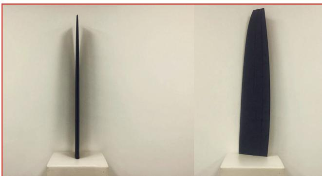
carbon. LEHVOSS has created the formulation that satisfies the structural requirements of the rudder for the Mini 650 very well.
