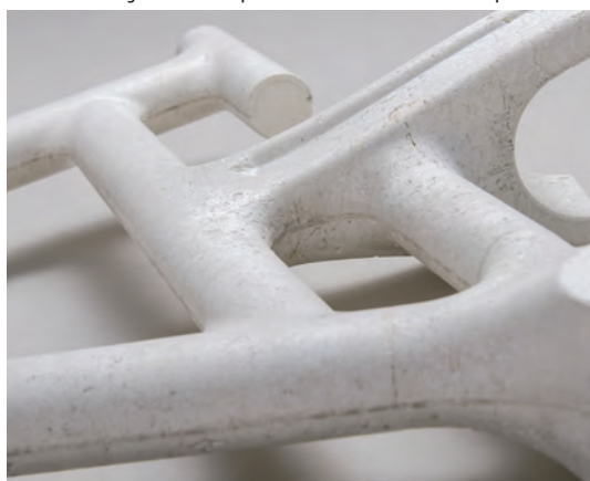
Fig. 1 Three-dimensional complex core made with Rohacell® Triple F Anima 3D dalla geometria complessa realizzata con Rohacell® Triple F
