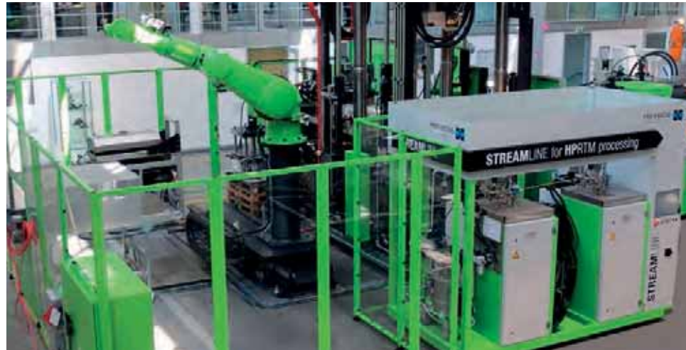
HP-RTM machinery Macchinario HP-RTM Foto courtesy: Engel, Austria
