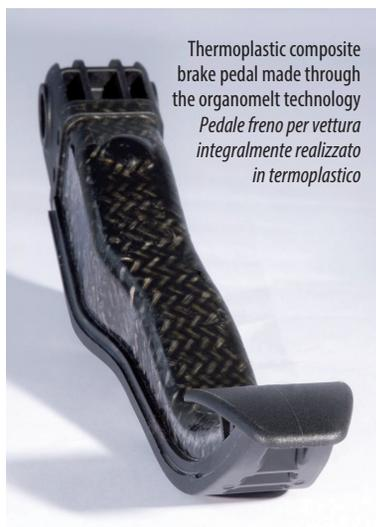
technology, are heated in an infrared oven, pre-moulded in the mould installed in the injection press and immediately overmolded with polyamide resins to create fasteners and ribs. The highly automatized plant manufactures components ready for assembling which do not need any open time. This allows to achieve the highest productivity rate, as the traditional metal brake pedals cannot be
