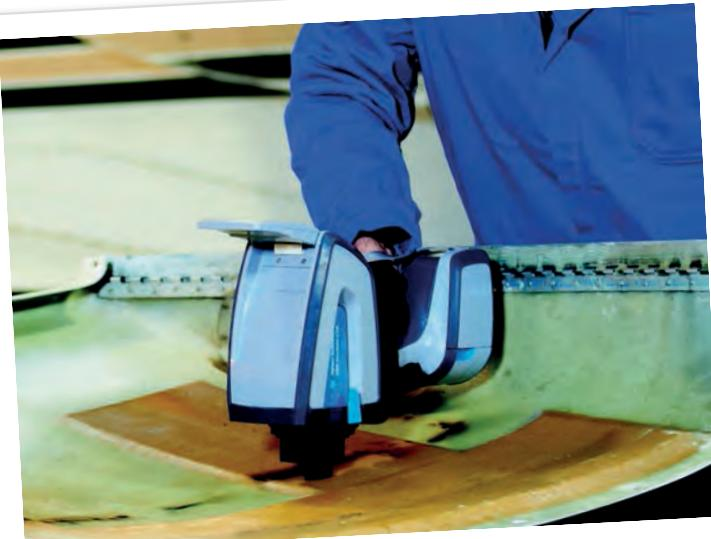
Fig. 1 - The Agilent 4300 handheld FTIR spectrometer equipped with diffuse reflectance sample interface weighs approximately 2.2 kgs
